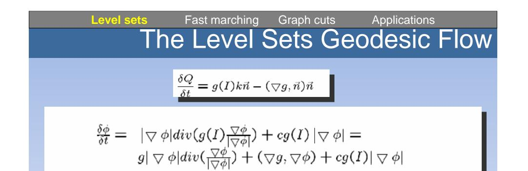
i.e. the level sets move according to:  $Q_t = g(I)(c+k)\vec{n} - (\nabla g, \vec{n})\vec{n}$
