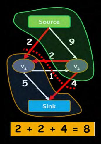
An st-cut (**S**,**T**) divides the nodes between source and sink.
