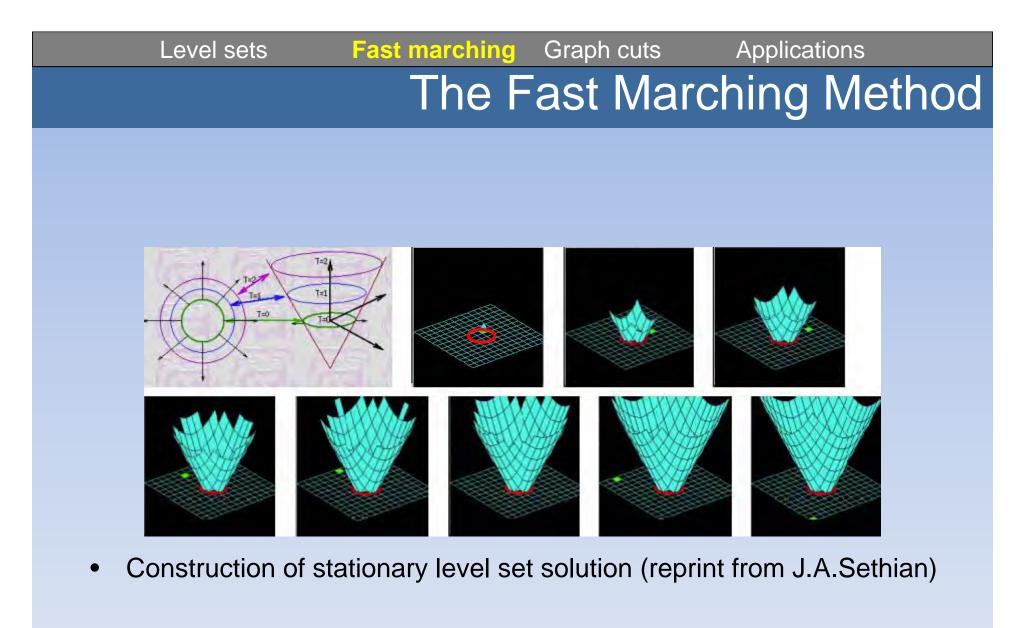
The fast marching level set method solves the general static Hamilton-Jacobi equation applied to a convex non-negative speed function.
