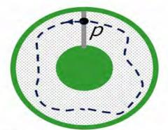
Compute the *shortest path p*->*p* for a point *p*. Repeat for all points on the gray line. Then choose the optimal contour. Graph Cuts approach
