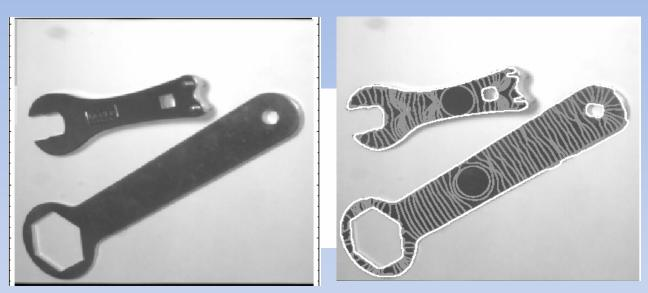
Outward motion to detect close objects. The initial contour is given by the image frame
